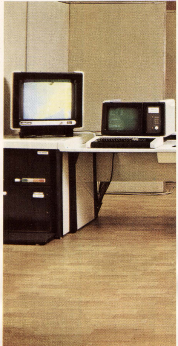
Hardware system for digital image analysis
